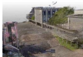
Point cloud data measured by Terrestrial Laser Scanner (Visualized by RGB values)
