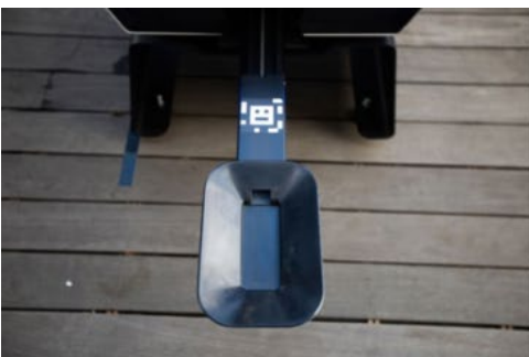
Skydio X2's bottom-mounted battery slide
